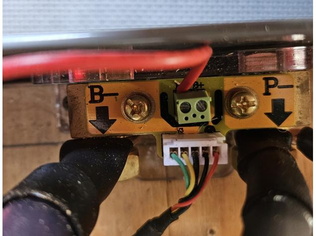
The large black wires are 1/0 gauge passing through the shunt to the battery.
