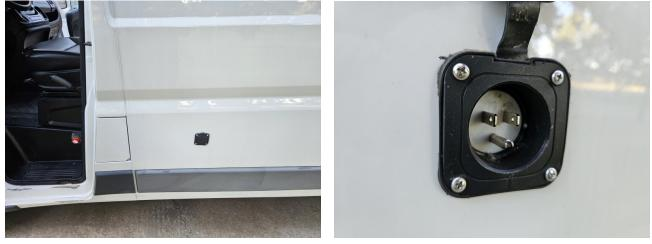
This inlet supplies power to an outlet strip mounted below the countertop surface.
