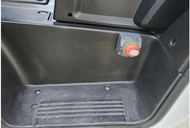
From **Switch #1**, the positive cable attaches to the back side of the Renogy 60A DC to DC charger.
