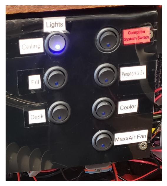
For best results, when powering up the computer, turn on the Peripherals switch first, wait about fifteen seconds, then turn on the Computer System power switch. The computer will automatically boot.
