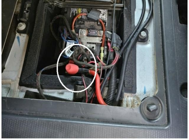
The cable runs under the step panel to **Switch #1**. Only position #1 is active in this switch.
