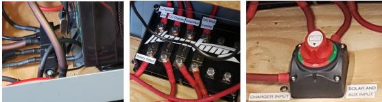
Position #1 selects the vehicle engine charging option while Position #2 selects Solar and Aux input. The selection between Solar and Aux is made through **Switch #4** and will be discussed later.
